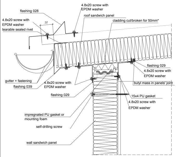
\* in case of breaking the cladding, max lenght of bracket 300mm
