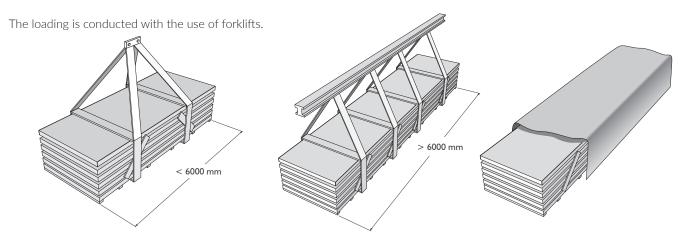
Unloading should also be conducted with the use of forklifts. In case of unloading with the use of cranes, webbing and trawl boards should be used, and for the packets longer than 6 meters the use of a transverse beam is necessary. The trawl boards should stretch the webbing over and under the packet.
