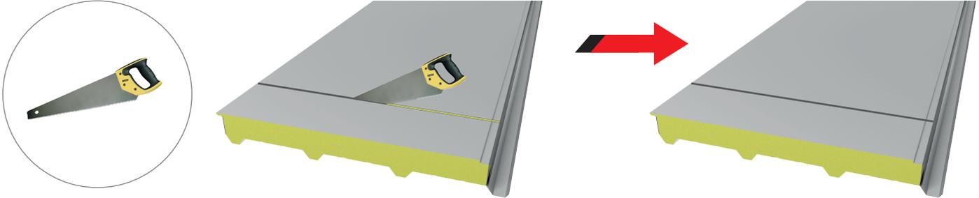
**2** Using the cutting set with wire, cut the PU in the horizontal way to the edge of the panel and remove the insulation including the internal facing.
