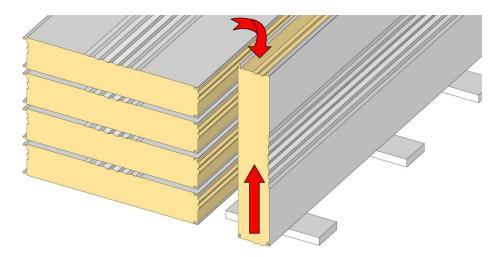
**Lightly moisten** the foam surface on the joint with a damp sponge (over the entire length of the panel) to improve the adhesion of the foam applied. Do not allow the water jet to remain on the joint surface - the joint should be moist, not flooded with water.
