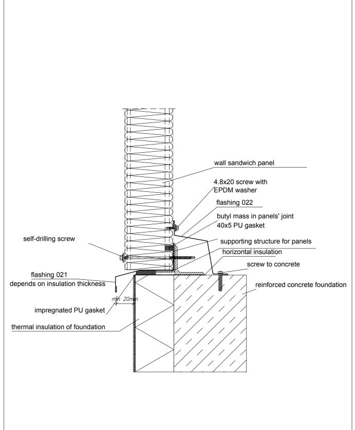
Flashings' fastening - screws (rivets) every 300 mm.
