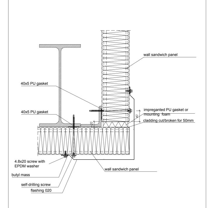
Flashings' fastening - screws (rivets) every 300 mm.
