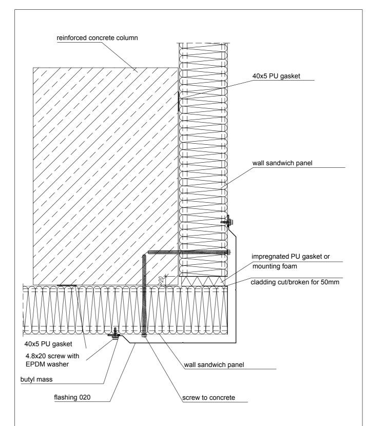
Flashings' fastening - screws (rivets) every 300 mm.
